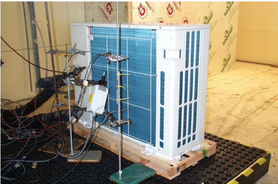
Figure 2 Heat pump in BRE heat pump test chamber prior to application of coil coating
